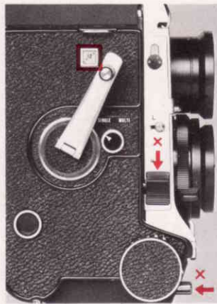
(4) When the last film in roll is exposed (after 12 or 24 exposures).
